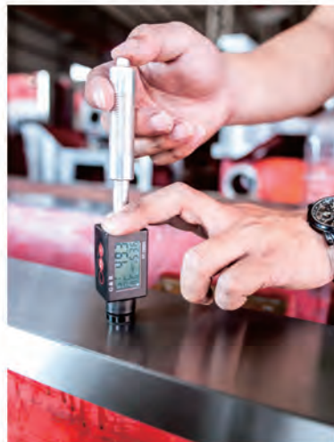
Measurement of inspection for hardness
